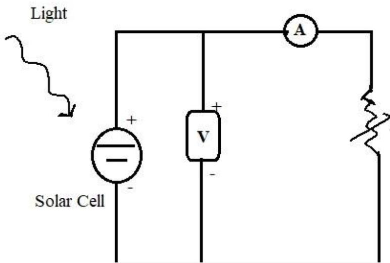
Fig.1 Circuit Diagram to measure the current-voltage characteristics of a solar cell
