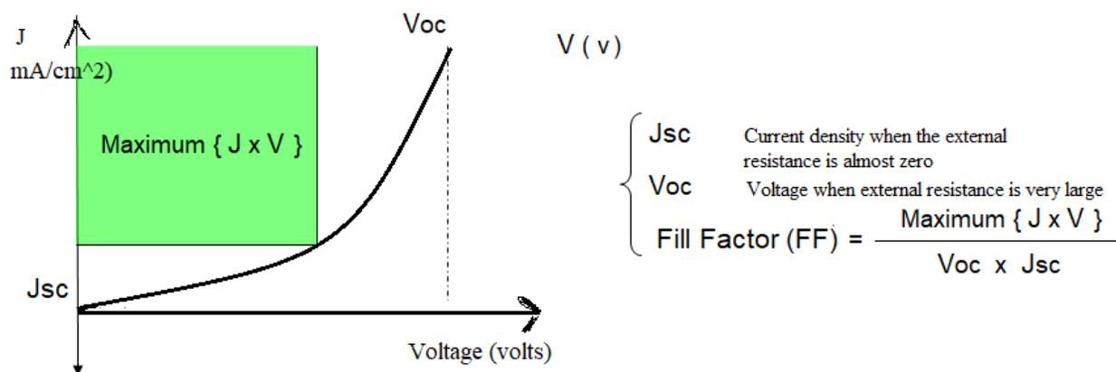
Graph of current density vs. Voltage. The fill factor (FF) is the ratio of the area of the green rectangle to the area formed by the dotted line.
