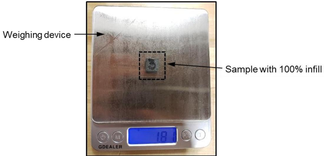
**Fig.6** Weighing device measuring the sample with 100% infill
