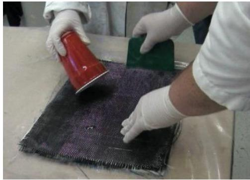
4. Start pouring or applying the epoxy immediately, the larger the quantity of mixed material in the cup the faster the Pot-life and working time.
