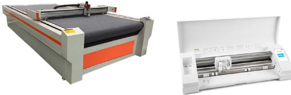
Figure 3: Industrial CNC knife with 160cm wide bed (left, stylecnc.com), and consumer die cutter with 30cm wide rollers (right, silhouetteamerica.com). Both show a drag knife on a gantry.
