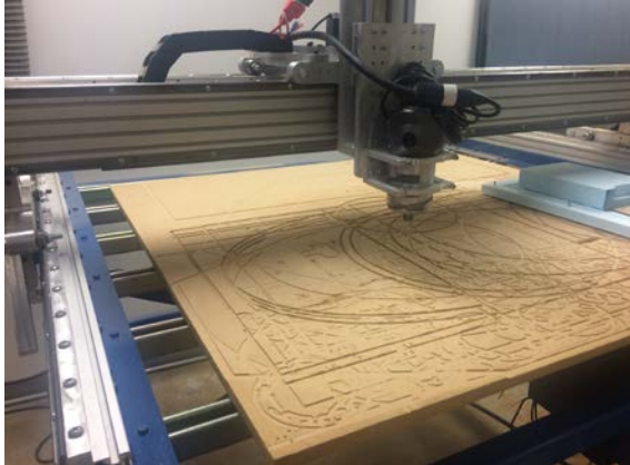
Figure 5: This CNC machine work surface, in the middle of the image, is level but uneven due to use of other cutting tools on it. The bar across the top of the image is the gantry, and the dark object it is holding on the right is a router, which is ready to be removed and replaced with a knife. To perform as a CNC knife, the work surface of this setup needs to be routed smooth or fully replaced.
