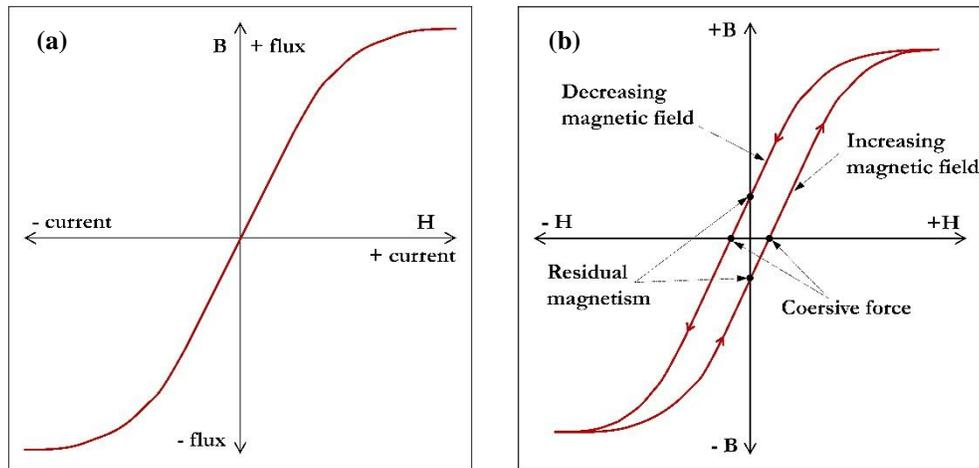
**Fig. 2** Typical B-H curve shows the the increase in magnetic field results to increase in magnetix flux, (a) B-H curve, (b) the difference in B-H curve when the magnetic field is applied and removed in practice [3].
