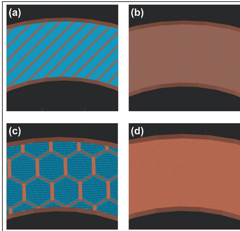
**Fig. 4.** Horizontal cryosections of transformer cores with different infill patterns and percent fill. (a) Rectilinear pattern with 20% infill density, (b) rectilinear pattern with 100% infill density, (c) honeycomb pattern with 20% infill density, (d) honeycomb pattern with 100% infill density.
