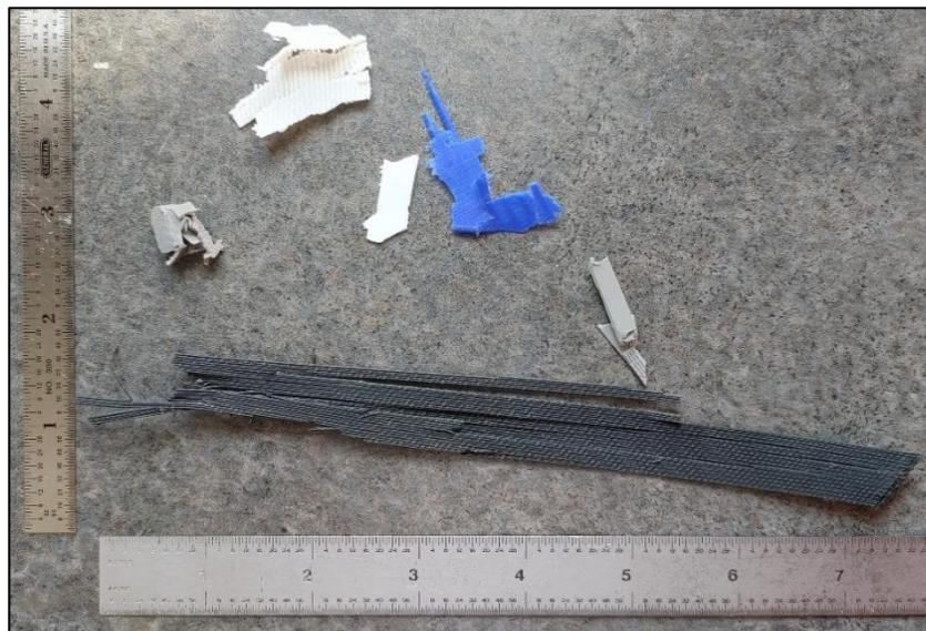
**Figure 2.2:** These previously shredded materials are still too large to be used for extrusion. Again, the pieces are greater than 5mm or 2/10ths of an inch in all dimensions of Length x Width x Height.
