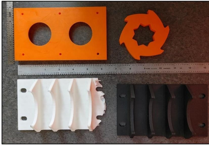
**Figure 2.1:** These failed prints are too large to be used for extrusion. The pieces are greater than 5 mm or 2/10ths of an inch in all dimensions of Length x Width x Height.
