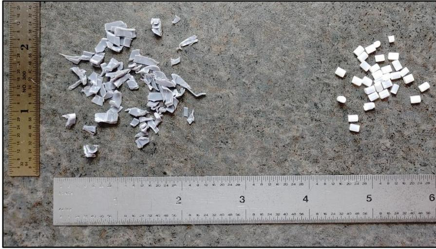
**Figure 2.3:**(Left) These previously shredded materials are acceptable for use in the extruding process. The pieces are under 5mm or 2/10 in. in all dimensions and are consistent in sizes.
