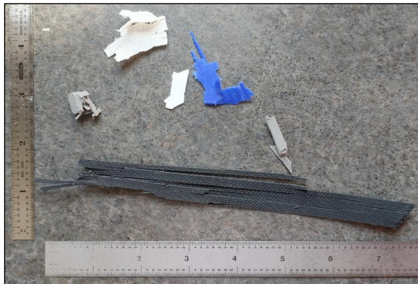
Figure 2.1: These failed prints are too large to be used for extrusion. The pieces are greater than 5 mm or 2/10ths of an inch in all dimensions of Length × Width × Height.
